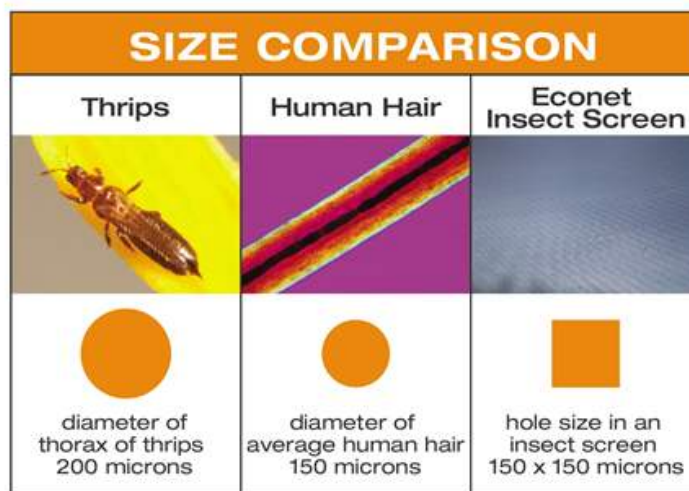
Figure 1: A size comparison of thrips, human hair and screen hole size.
