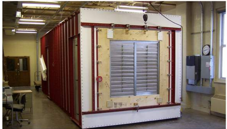
Figure 3: Wind tunnel used for evaluating airflow performance of screens.
